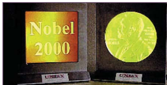
Polymer LEDs made by Gang Yu, 5" x 5" and 5.1" diameter, to commemorate the 2000 Nobel Prize. These single pixel polymer LEDs are fixed digital images with a resolution of 80 dpi. (Courtesy of Alan Heeger and Gang Yu of DuPont Displays.)
