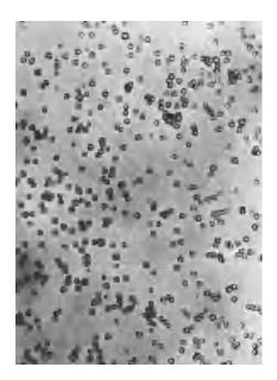
Figure 7. Sea-water microspheres. These are stable at pH 9. About 1 µm in diameter.
