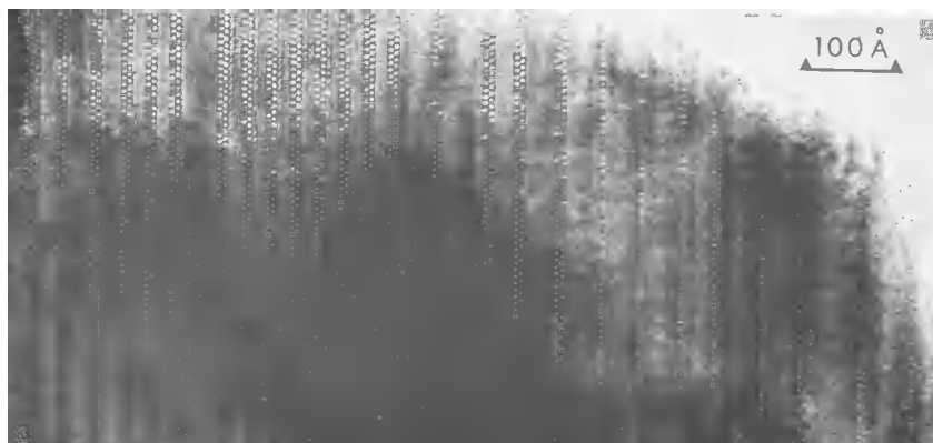
Fig. 13. Image of disordered structure of rubidium intergrowth tungsten bronze.
