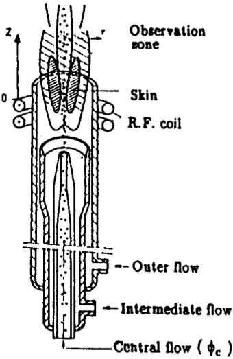
Fig. 3<sup>a</sup>. A sketch of an ICP
