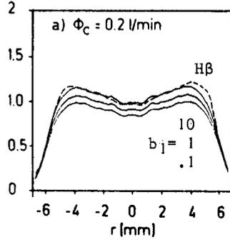
Fig. 3<sup>b</sup>. Density measurements as measured by absolute line intensity method and by H $\beta$ -broadening [18]
