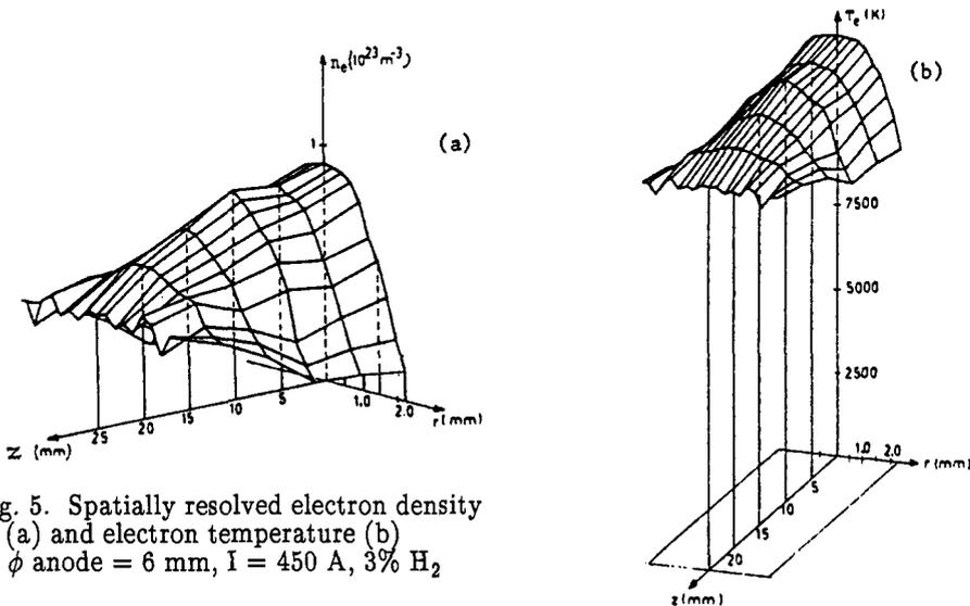
Fig. 5. Spatially resolved electron density (a) and electron temperature (b)
