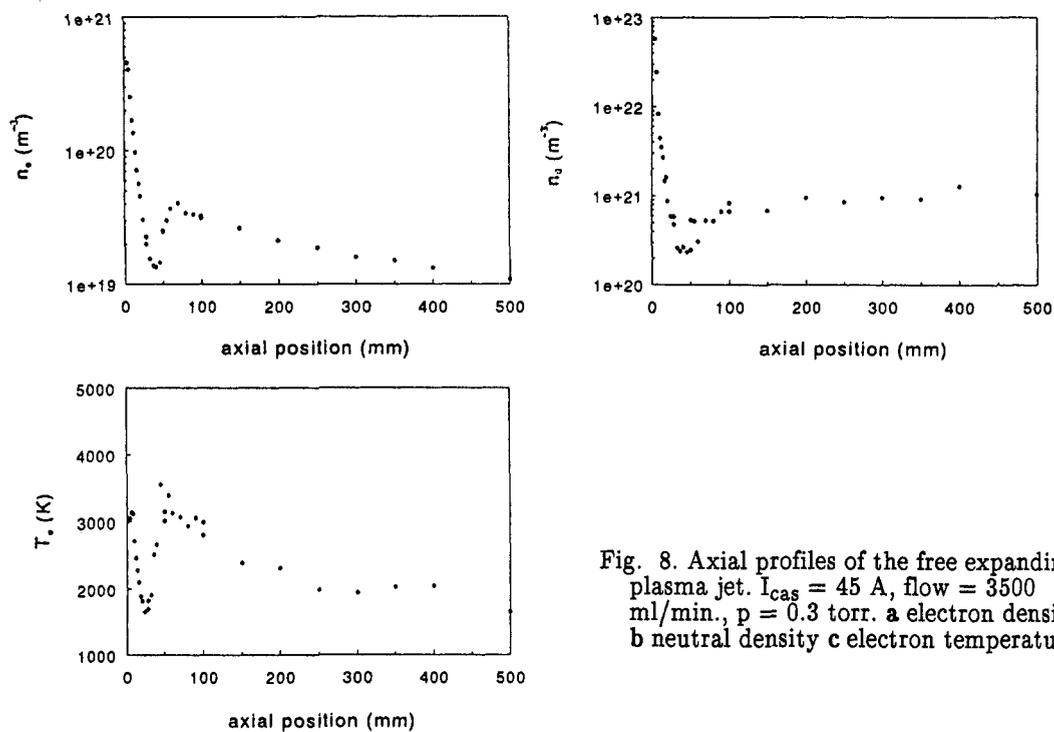
Fig. 8. Axial profiles of the free expanding plasma jet.  $I_{cas} = 45$  A, flow = 3500 ml/min.,  $p = 0.3$  torr. a electron density b neutral density c electron temperature
