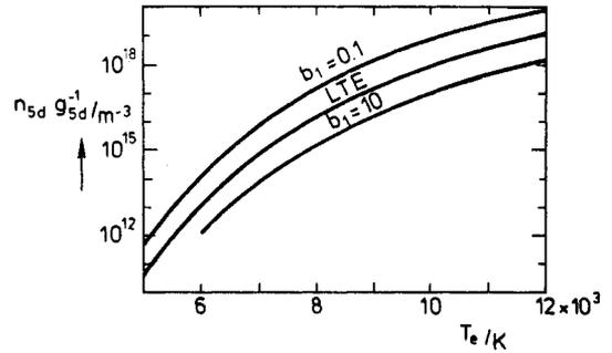
Fig. 1<sup>b</sup>. The relation between  $n_{5d}/g_{5d}$  and  $T_e$  with  $b_1$  as parameter  $g_{5d}$  [2]
