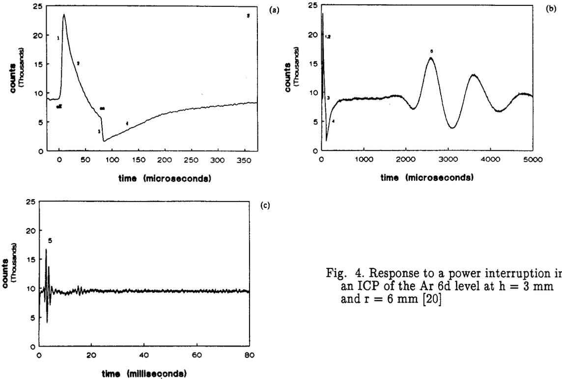
Fig. 4. Response to a power interruption in an ICP of the Ar 6d level at  $h = 3 mm$  and  $r = 6 mm$  [20]
