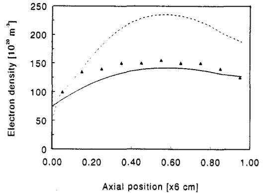
Fig. 7. Measured (.) and calculated electron densities (dashed line, peak value, full line: average value) [25]
