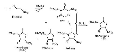
Scheme 10 Reaction leading to ring closure of anti and syn adducts.
