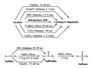
Fig. 2 Oxidation of alcohols to carbonyl compounds and oxidation of sulfides to sulfoxides and sulfones. (Reproduced with permission from R. S. Varma, *McGraw-Hill 2002 Year Book of Science and Technology*,
