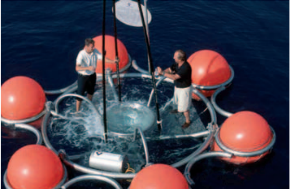
Platform of fresh water capture Nymphaea Water – Aubagne - France
